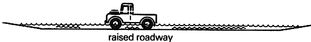
Figure 21(b). Wide crossing, shallow flood.
